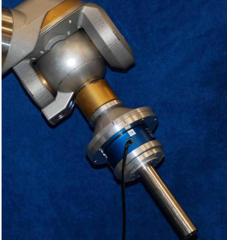
Figure 3.11: 1 kg Cylindrical Mass Attached to FTS
