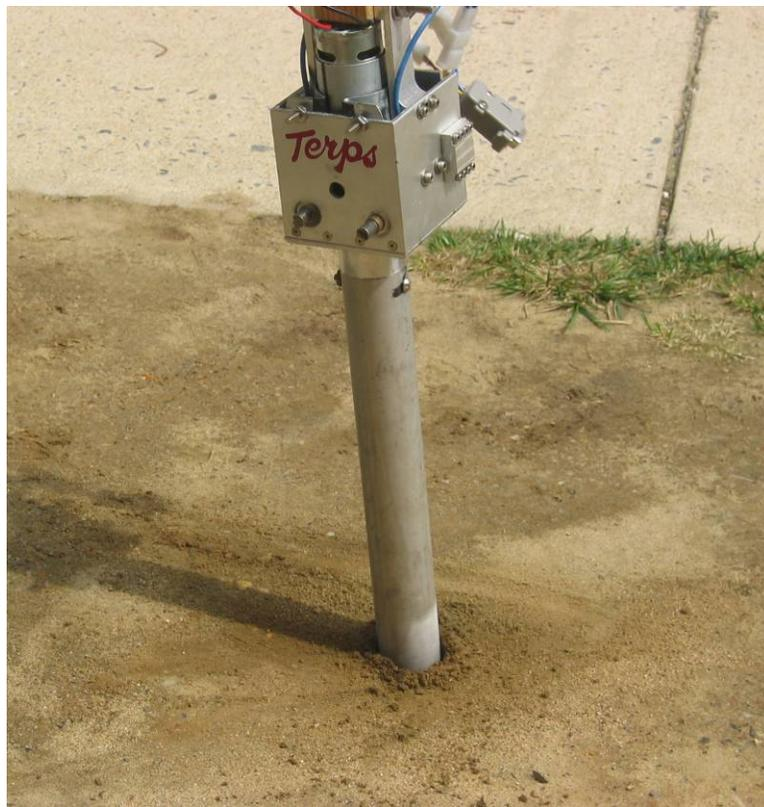
**Figure 7-5: TERPS Collecting a Soil Core (scoops not attached)**
