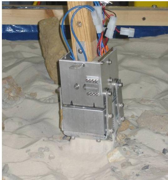
**Figure 7-3: TERPS Sifting Soil Sample**
