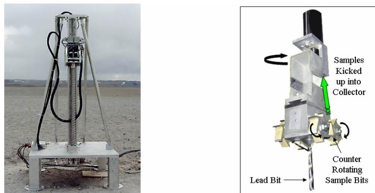
**Figure 2-11: Honeybee Robotics Sampling Systems**
