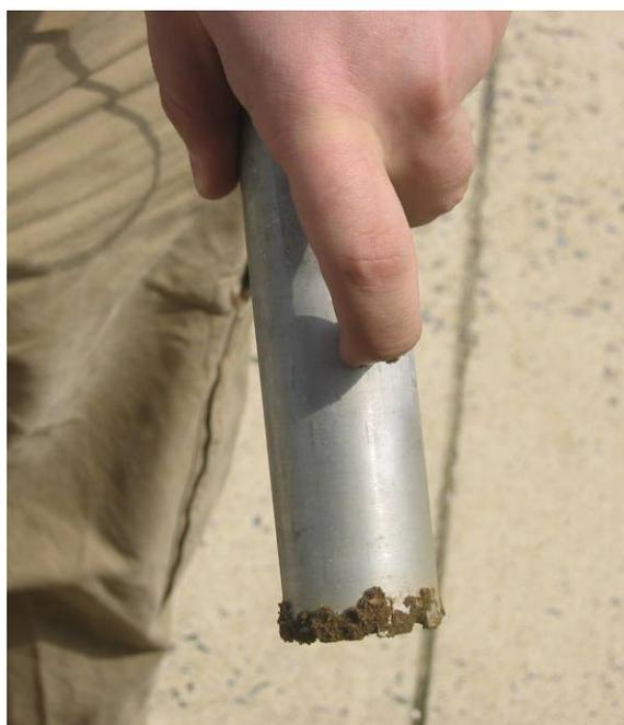
**Figure 7-6: 4 cm Soil Core**
