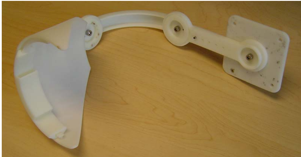
Figure 8: Singular configuration for prototype I
