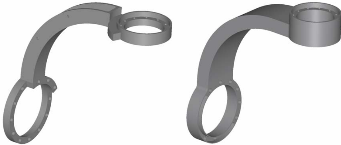
Figure 40: Original shoulder link design (left) and modified shoulder link design (right), which connects the first shoulder joint with the second shoulder joint
