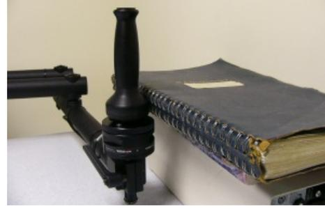
Fig. 7: Detecting the edge of a spiral notebook during a tele-assessment test.
