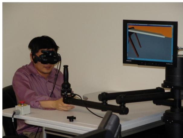
**Fig. 1:** Subject performs virtual beam task with *InMotion2 Robot* while donning stereographic goggles.
