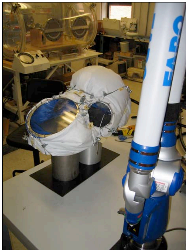
Figure 6: A preliminary MUT configuration to approximate the geometry of the MX-2 HUT.
