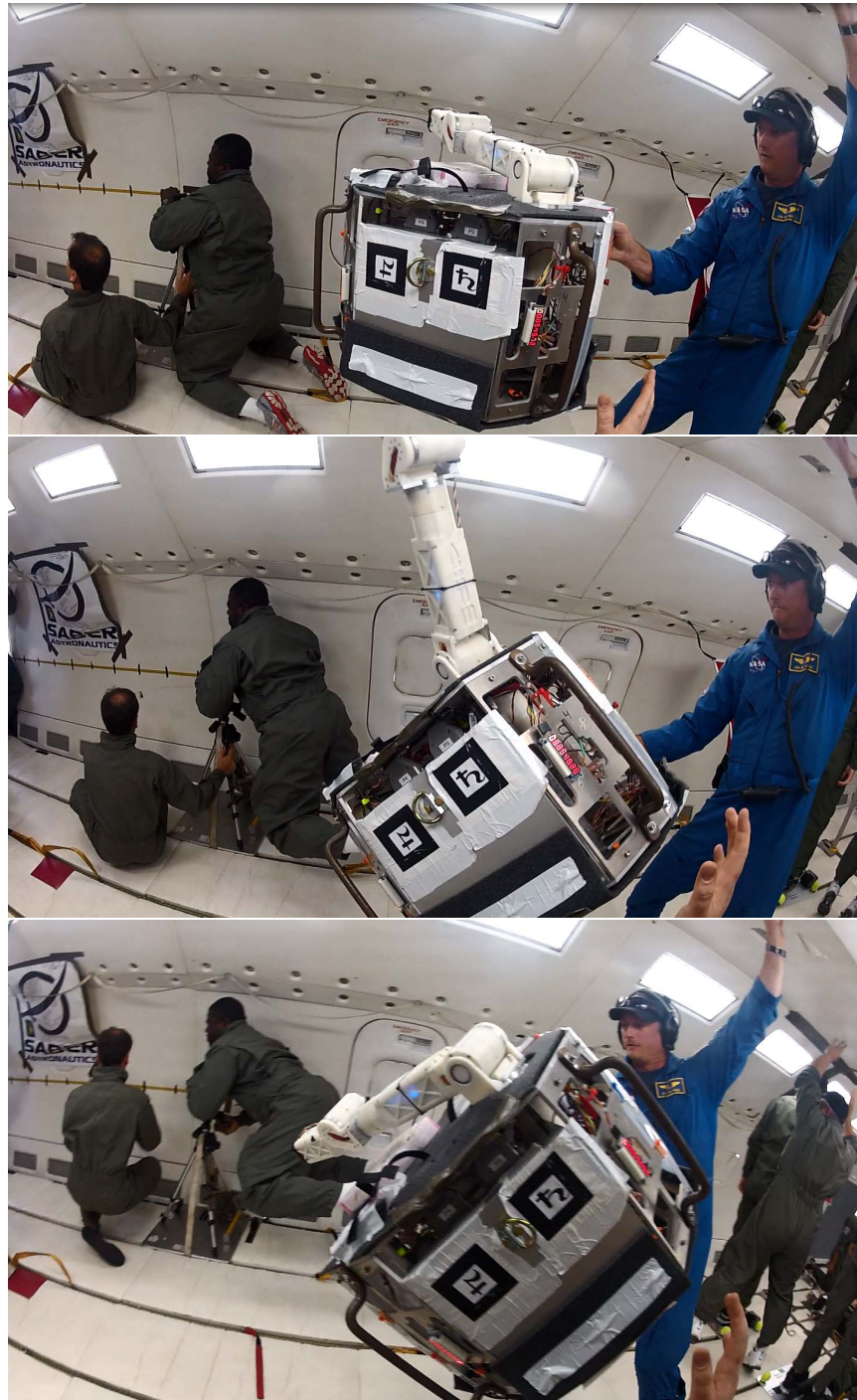
Figure 4.24: Flight 2, Parabola 3: Free-flier at release of fast pitch maneuver (upper), at the halfway point at 130 degrees from starting position (middle), and at the end of the maneuver (lower). The base has significantly rotated about a coupled axis during the single maneuver, three identical motions of the manipulator were performed during this parabola.
